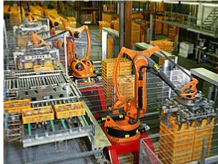
KUKA industrial robots being used at a bakery for food production
